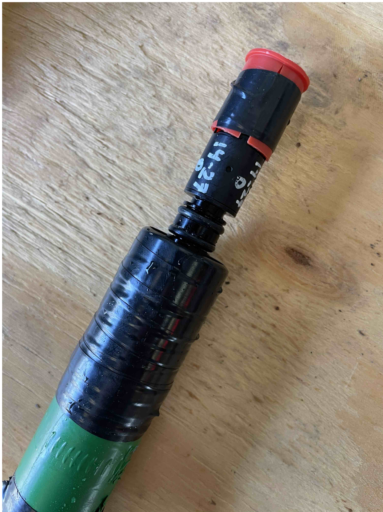
Fig. 4: Flooded chipod with sensor separated from pressure case.
