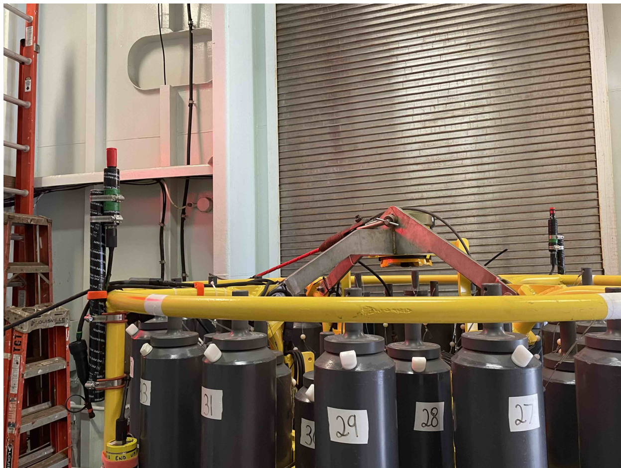
Fig. 1: Upward-looking chipod sensors attached to the rosette.
