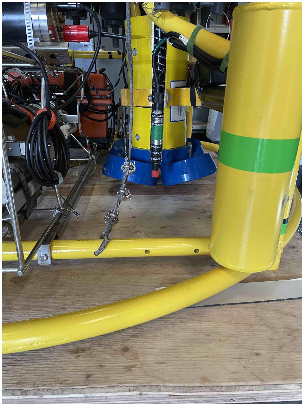
Fig. 2: Downward-looking chipod sensor attached to the rosette.
